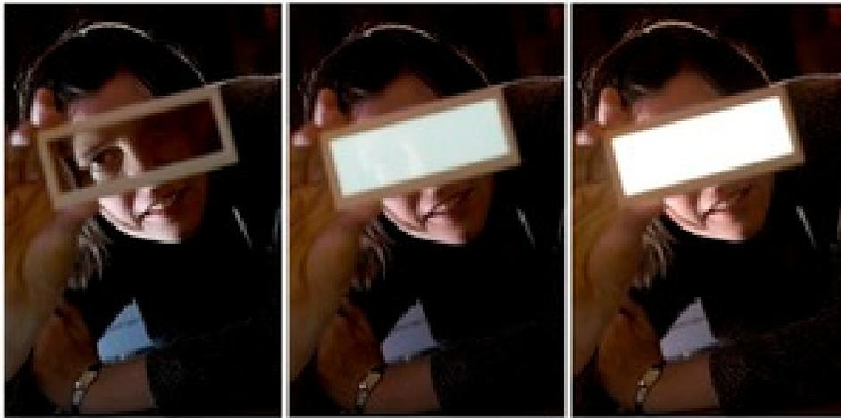
OLEDs are very power efficient and they can be made very thin. An OLED light bulb is actually a thin film of material that emits bright white light. Because OLEDs can be flexible, or even transparent, there are a huge number of new OLED lamp designs possible.
